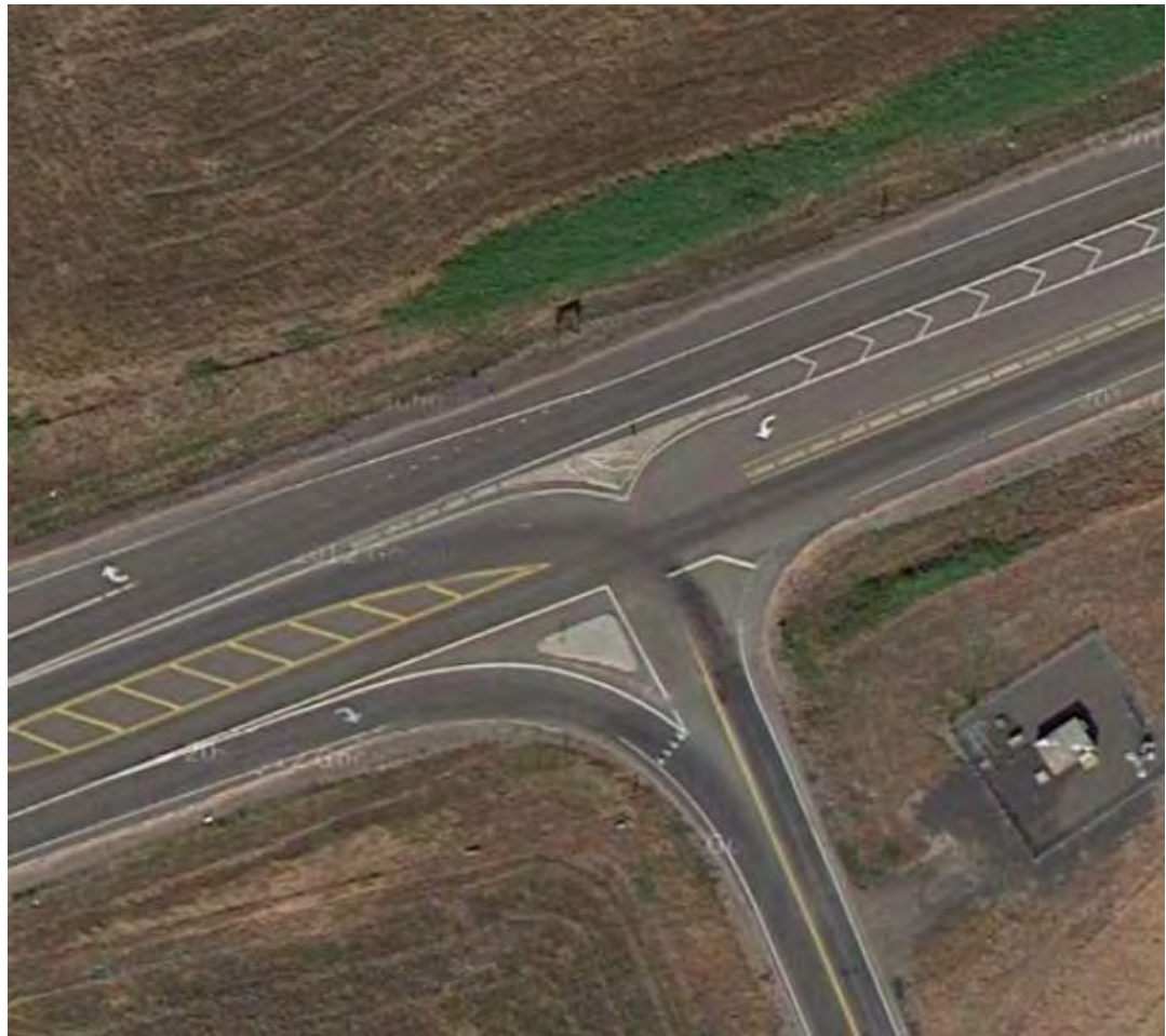
Figure 5-6: Two-stage left-turn treatment (Aerial imagery of Salmon River Highway and SE Cruickshank Road intersection in McMinnville, Oregon).
